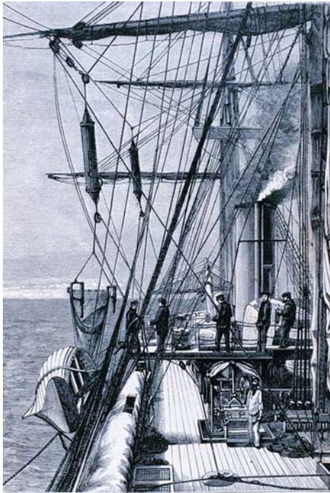
FIG. 17.—The Dredging and Sounding Arrangements on board the 'Challenger.'
