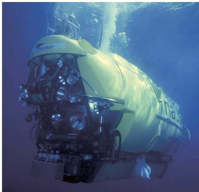
The Nautilie , launched in 1984, is one of the few manned submersibles that can descend to 6000 m water depth. It is capable of exploring 97 % of the world's ocean floors. © Ifremer/Eric Lacouppelle
