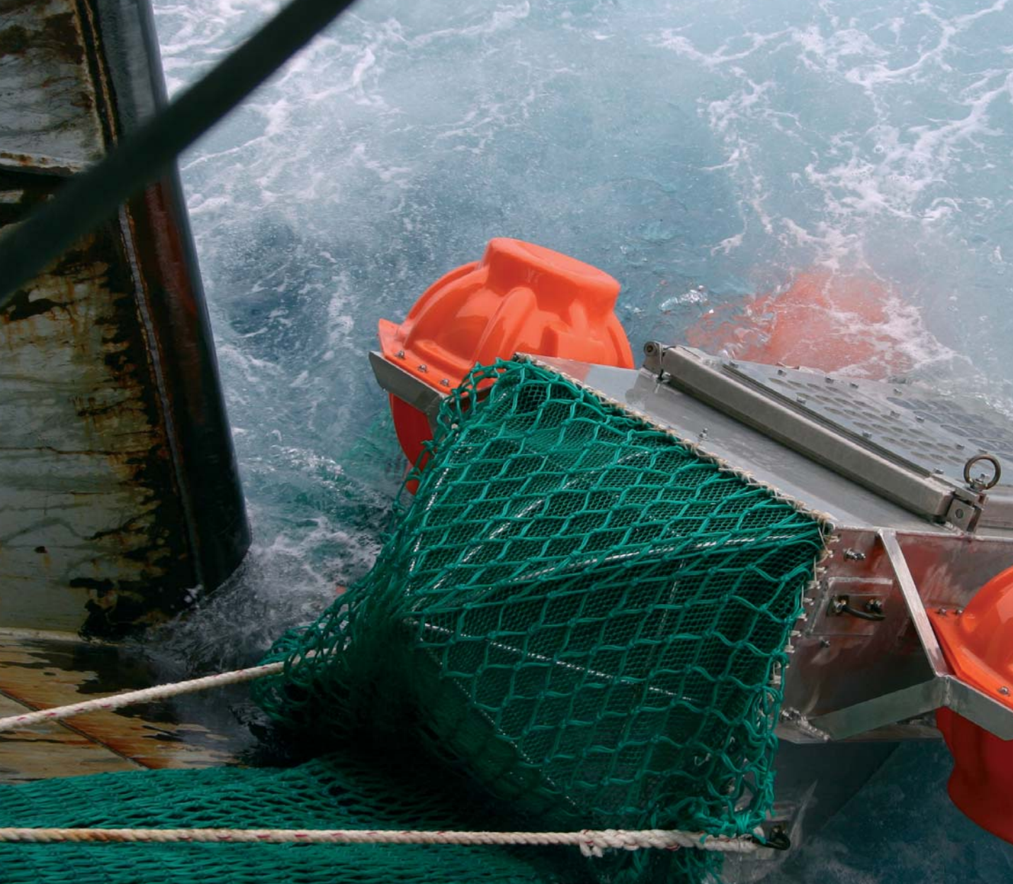
The cod-end aquarium being retrieved. The aquarium helps keep specimens in good condition. It also has an internal digital video camera. © MAR-ECO
