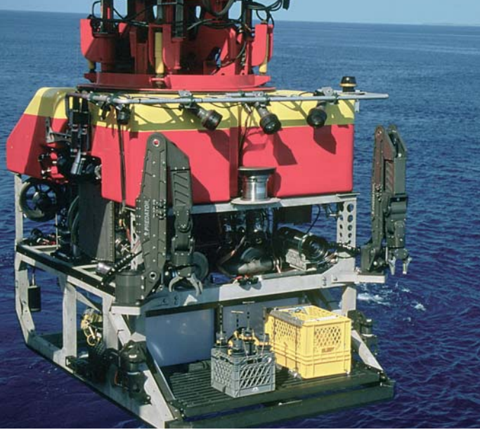
The Remotely Operated Vehicle (ROV) Isis with the ability to explore the seabed down to 6500 m. © National Oceanography Centre, Southampton
