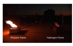
Figure 6 - Hydrogen and Propane Flames at Night (Photo courtesy of ImageWorks)
